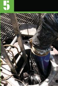
an umbilical line that can be as long as 300 feet. The line is attached to the life support trailer, where the console operator monitors and controls the elaborate air delivery system.
